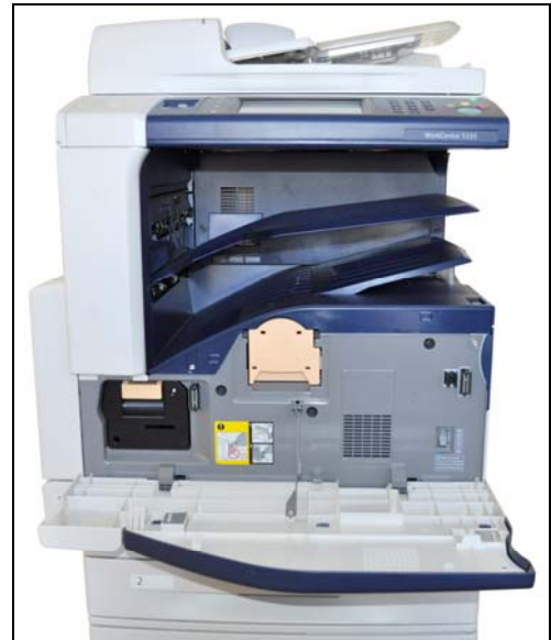
Above and below: In order to replace the Xerox WorkCentre 5335's toner cartridge the user must first open the device's front cover by pulling this panel door down. Once the door is open the user then simply slides the toner cartridge out for replacement.
