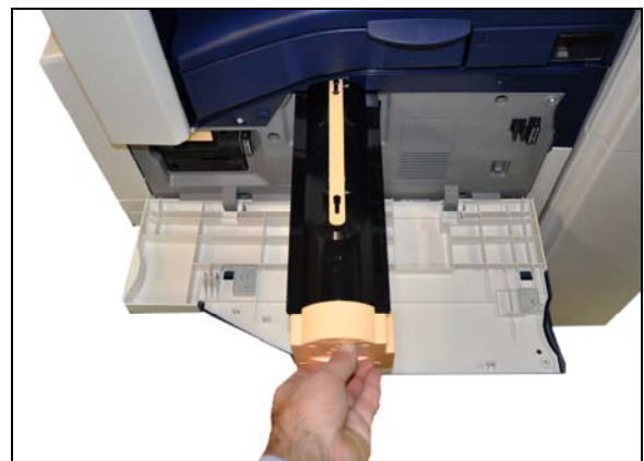
Above and below: In order to replace the Xerox WorkCentre 5335's toner cartridge the user must first open the device's front cover by pulling this panel door down. Once the door is open the user then simply slides the toner cartridge out for replacement.
