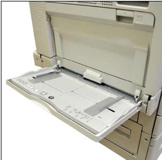
Above: The 50-sheet bypass tray can be adjusted by sliding the gray levers into place. The feeder can be adjusted for envelope printing.
