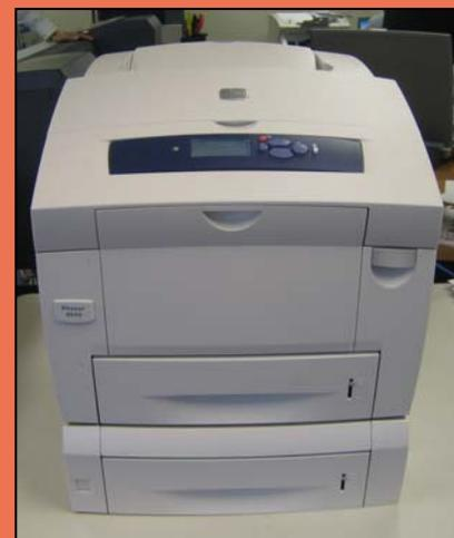
The Xerox Phaser model 8560DT tested by BERTL was equipped with an additional 525-sheet paper drawer, two-sided output capability, 512 MB of memory, and a 40-GB hard drive.
