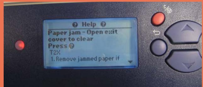
A flashing red LED on the control panel alerts users that the printer is in need of attention.
