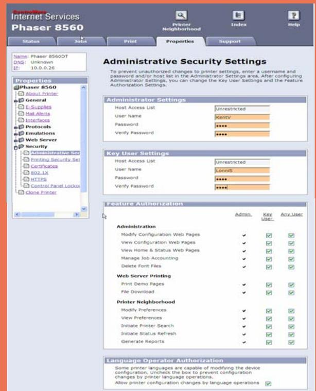
Setting up security settings protects the device from being configured or changed without authorization.
