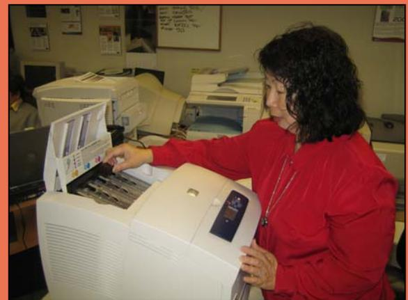
The BERTL analyst performs routine management on the Xerox Phaser 8560. Solid ink sticks can be easily inserted into their proper color slot, which accommodates up to three sticks in each channel.
