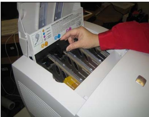
Users can easily replace the printer's solid-ink "sticks." To replace a stick, the user raises the top cover and drops the bullet in at the top of its channel. Up to three ink sticks can be placed in the channel at one time.
