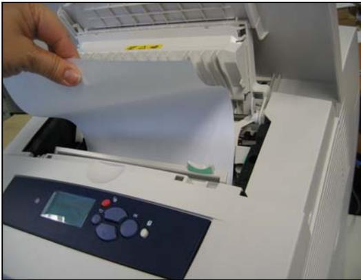
Most paper misfeeds can be easily removed from the front or near the top of the device. BERTL analysts did not encounter any problems or any hidden misfeed points.
