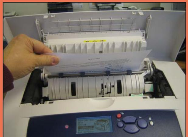
Removing paper misfeeds from the top exit cover is straight forward and easy to do. The control panel displays helpful animated graphics, and help information is readily available by pressing the “?” help key on the control panel.
