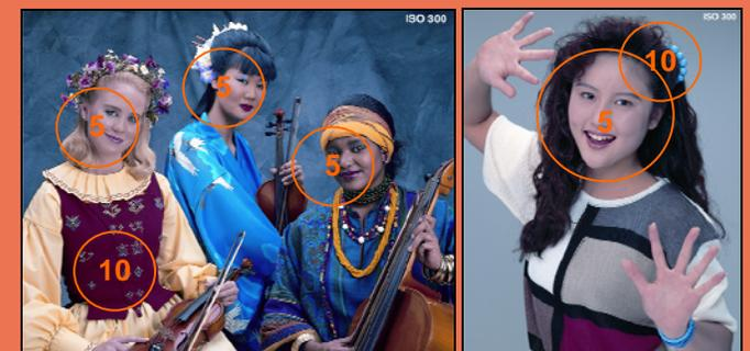
BERTL uses synthetic (photographic) test images obtained from ISO International Standard 12640--Graphic Technology--Prepress digital data exchange--CYMK standard color image data (CYMK/SCID) in order to evaluate the ability to print photographic images.
