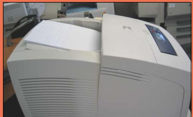
Print jobs are neatly output to the center default tray, providing a base for users to set up collated sets for post-process imposition such as saddle-stitch booklets or perfect binding.
