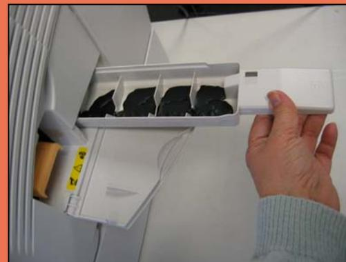
Most minor maintenance requirements for the Xerox Phaser 8560 can be performed in a matter of minutes including emptying the solid-ink waste tray, which is performed when a message appears on the control panel informing users that the waste tray is full.
