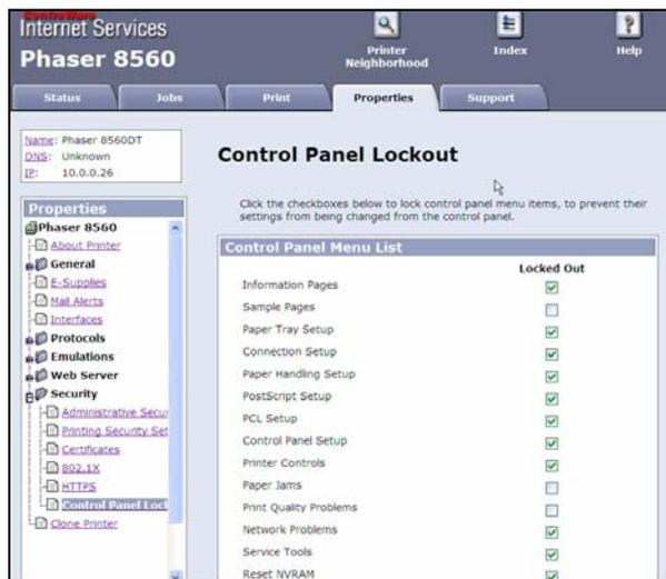
With the Phaser 8560, the administrator can enable control-panel lockout using Internet Services, so that unauthorized users can not change control-panel settings.
