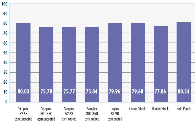
Based on BLI field testing of the Xerox Versant 80 with optional Performance Package. In BLI's media impact on productivity test, five sets of a 48-letter-image job are sent to the device and are output on different media types, with throughput time assessed between sets 2 and 5.
